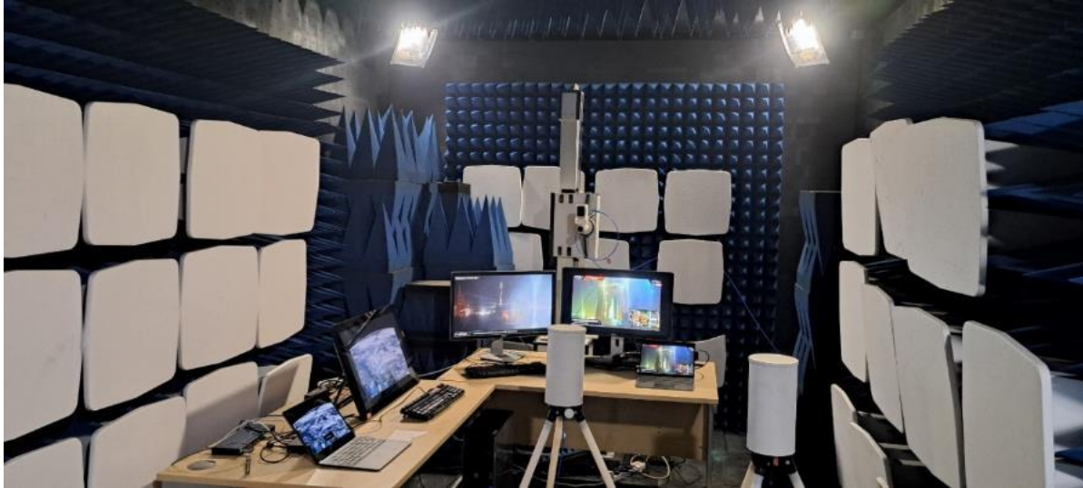
Figure 13: Mock office setup inside Ofcom's anechoic chamber at Baldock
