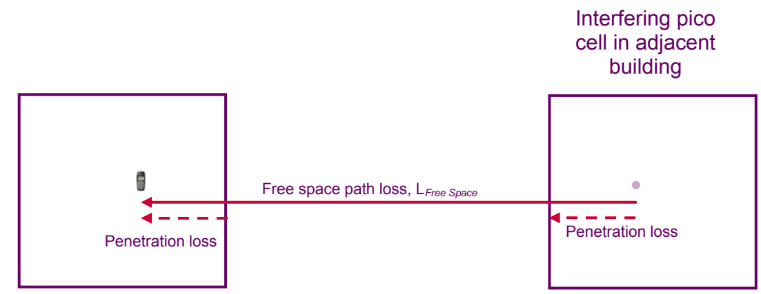
Figure E.4. Breakdown of the calculation of the transmission path of interferer
