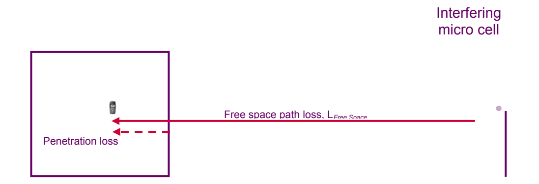
Figure C.5. Breakdown of the calculation of the transmission path of interferer
