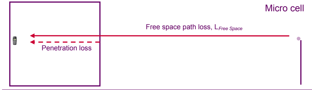
Figure C.2: Breakdown of the calculation of the transmission path of the wanted signal
