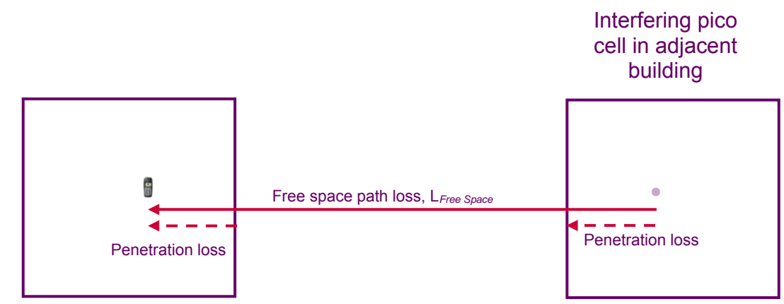
Figure B.3. Breakdown of the calculation of the transmission path of interferer
