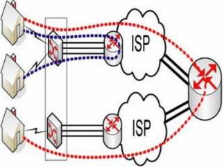
Bringing routing deeper into the network makes it ever more like a grid - which might be what we need to get the best out of technologies like peer-to-peer. Shorter distances means lower latency and lower lower jitter, and a much greater scope to use the capacity on the fixed price, uncontended portion of the network at zero extra cost.
