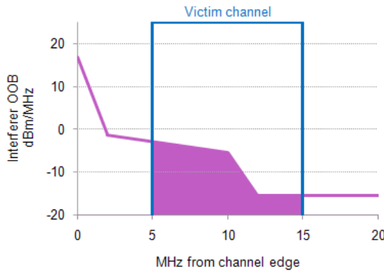
Figure A8.4: Interference power in the victim’s channel when victim and interferer channels are separated by 5 MHz
