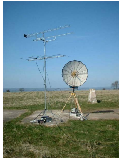
Portable Dish on Contest with VHF talkback
