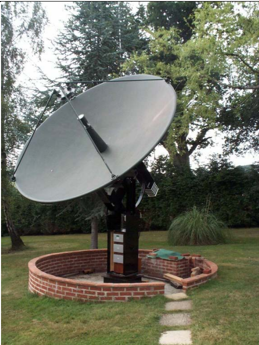
3400 MHz EME Moonbounce – with remote control computerised mount
