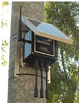
Figure 10: Installed Wasmote plug and sense. Source: Libelium
