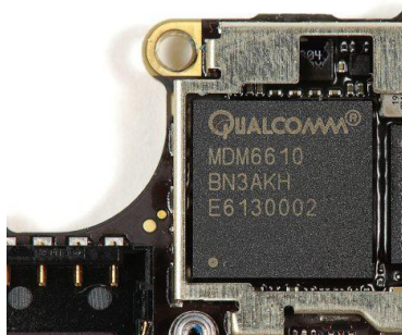
Figure 4.4: Apple iPhone 4S chip combining network GPS & GLONASS radios
