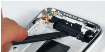
Figure 4.3: Apple iPhone 3G GPS antenna (being prised)
