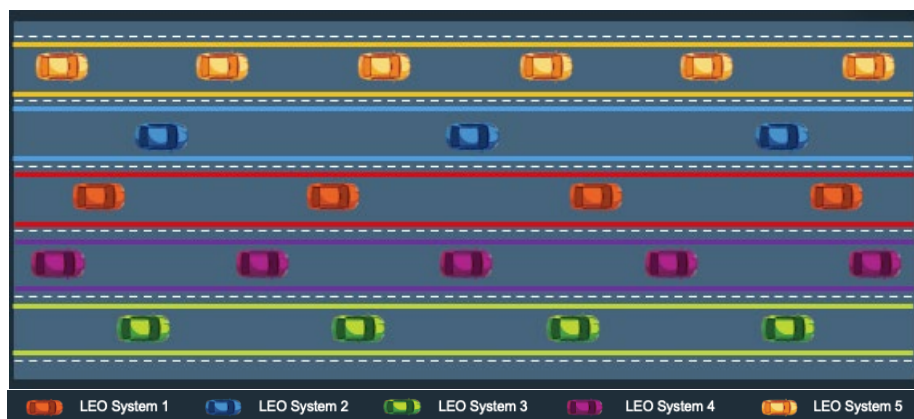
Figure 9: With reasonable orbital tolerances, many NGSO systems can share limited orbits.
