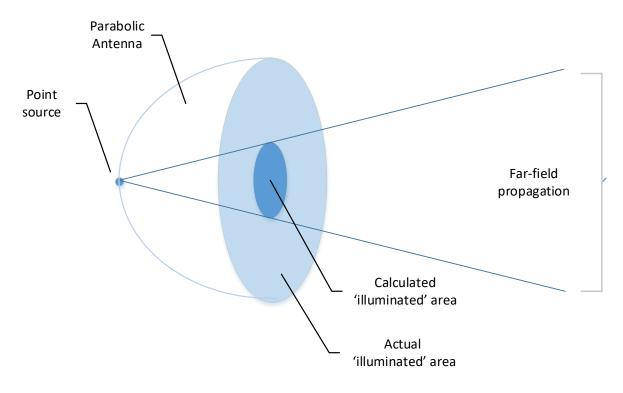
By way of example, consider a radiator operating at 80GHz, with a conducted transmit power of 0.1W and a 65cm parabolic antenna. At 80GHz, this antenna has a gain of 50dBi and a transmission beam-width of 0.45°. The radome is 30cm from the waveguide.
