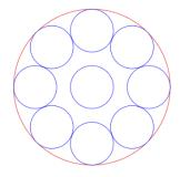
This alone shows the original Openreach 2.5 times 25mm fit in a 100mm duct to be at least highly pessimistic, or a result of poor engineering practice.
