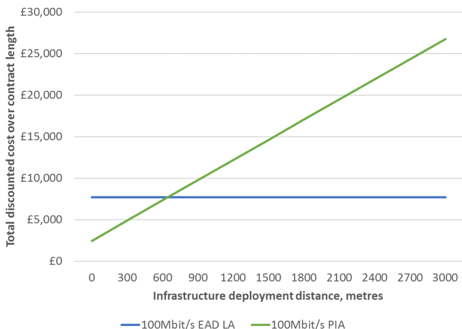
Figure 2: Five-year total cost of ownership, 100Mbit/s EAD LA versus own-fibre deployment using DPA (PIA)
