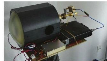
PHOTO 2: G8CUB's 288GHz receiver. Photo courtesy G4BAO.
