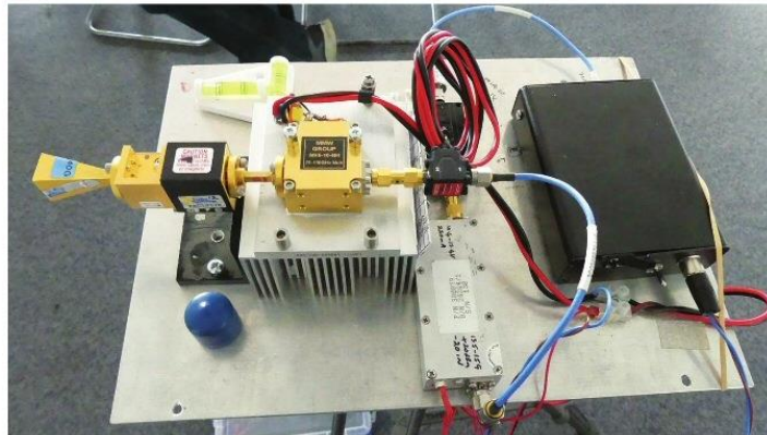
PHOTO 1: G8CUB's 288GHz transmitter. Photo courtesy G4BAO.
